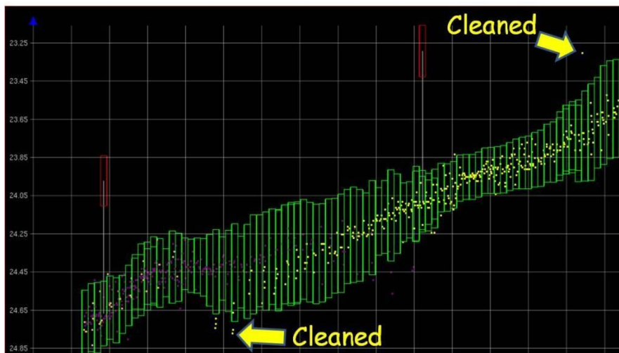
Figure 10: “Surface filter” tool is used to build a filtering screen around CUBE surface. Each filtering screen size can be adjusted based on nodes uncertainties or standard deviations. Soundings located out of filtering screen ranges are automatically cleaned
