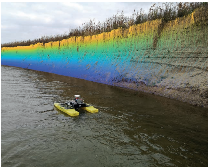
Fig. 3 Uncrewed water vehicle on a small river with LiDAR point cloud overlay on the river bank.
