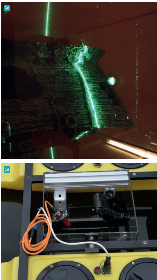
Fig. 4 Underwater laser light sheet triangulation system: (a) Laser line on a wreck model in a laboratory environment. (b) Sensor system mounted on the UUV.
