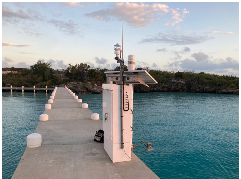
Fig. 2 Marine Environmental Monitoring Station at Sapodilla Bay, Turks and Caicos Islands. Remedial works was undertaken on the existing Sutron tide gauge, with installation of OceanWise's ip.buffer smart telemetry system, a meteorological sensor and GNSS leveling.
