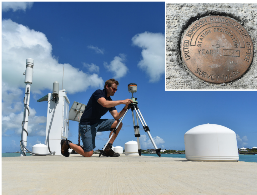
Fig. 3 GNSS leveling at Sapodilla Bay, Turks and Caicos Islands to establish geodetic benchmarks for tide gauge levelling and establishing a local datum.
