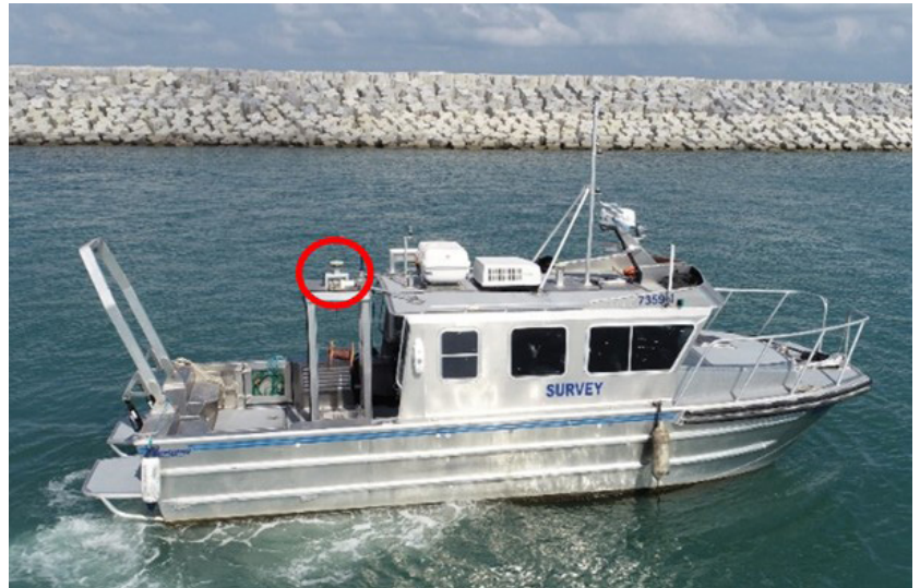
Fig. 2 The ADEL survey vessel. The GNSS antenna rigidly attached to the ship's hull is marked in red.
