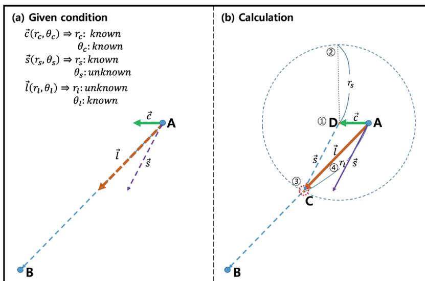
Fig. 4 Schematic diagram for procedures of calculating actual ship sailing speed  $r_l$  between A and C denote the direction of each vector. The circled numbers in (b) denote the sequence in which  $r_l$  is calculated.
