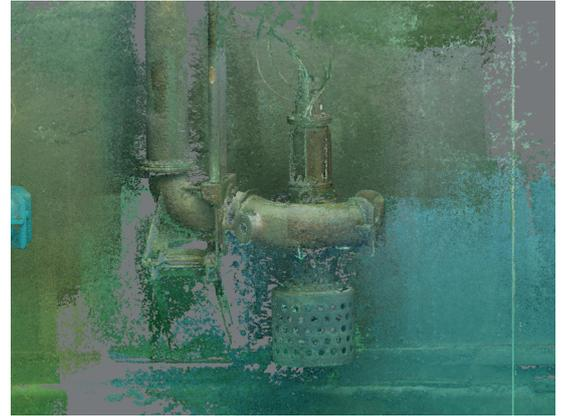
**Fig. 8** Calculated cylinder for the pipe in the point cloud of the water filter.
