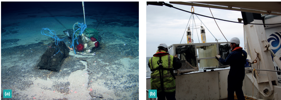
Fig. 7 Benthic landers including (a) mooring deployed with sunken wood and bone on a seamount on the South West Indian Ridge deployed during the IUCN – NERC Seamount Project, (b) fish trap deployed during The Nippon Foundation Nekton Ocean Census NIWA Bounty Trough Expedition, South West Pacific, 2024. Photos by IUCN – NERC Seamounts Expedition (a) and A. D. Rogers (b).
