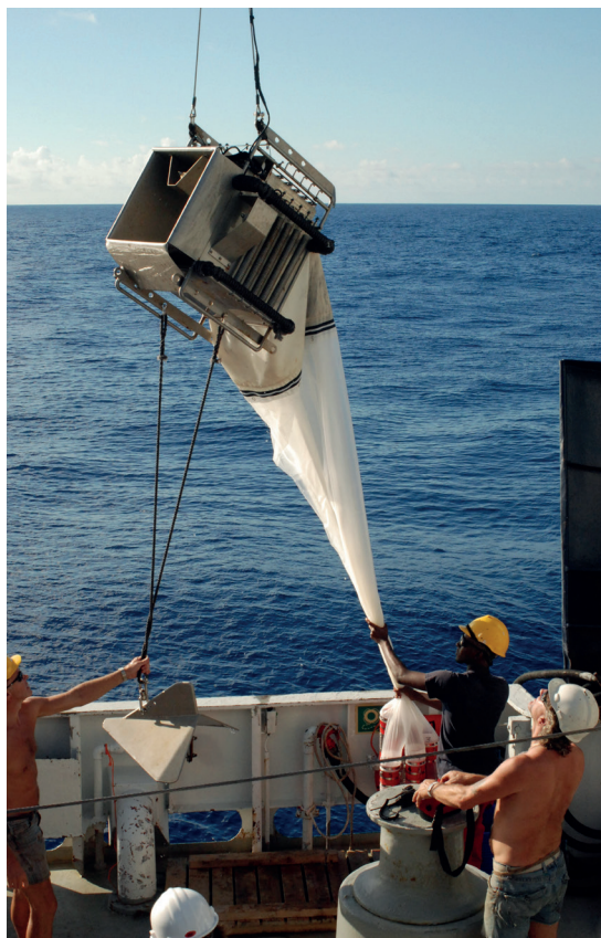
Fig. 3 Multinet being recovered after sampling microzooplankton on the Southwest Indian Ridge, southern Indian Ocean, 2009 during the IUCN – NERC Seamount Project. Photo by A. D. Rogers.
