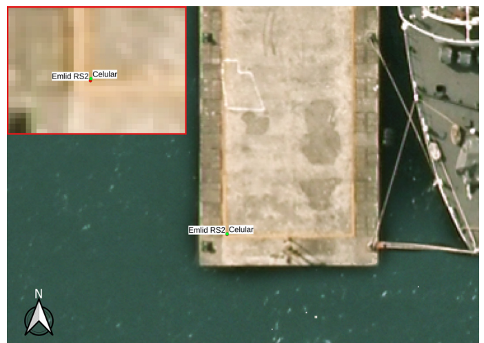
Fig. 10 Plotted coordinates of the PIRF point (Sirius – Pto Drone) using the ONRJ as a reference station. Source: Adapted from QGIS (2022).
