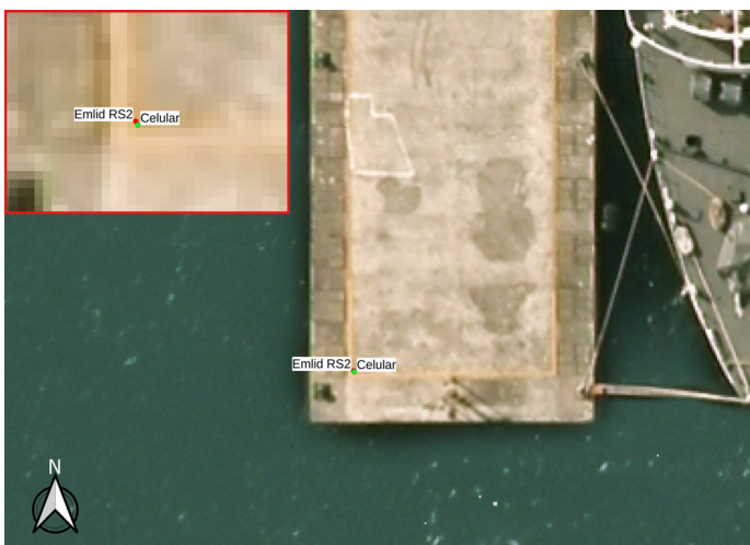
Fig. 9 Plotted coordinates of the PIRF point (Sirius – Pto Drone) using the RJNI as a reference station. Source: Adapted from QGIS (2022).
