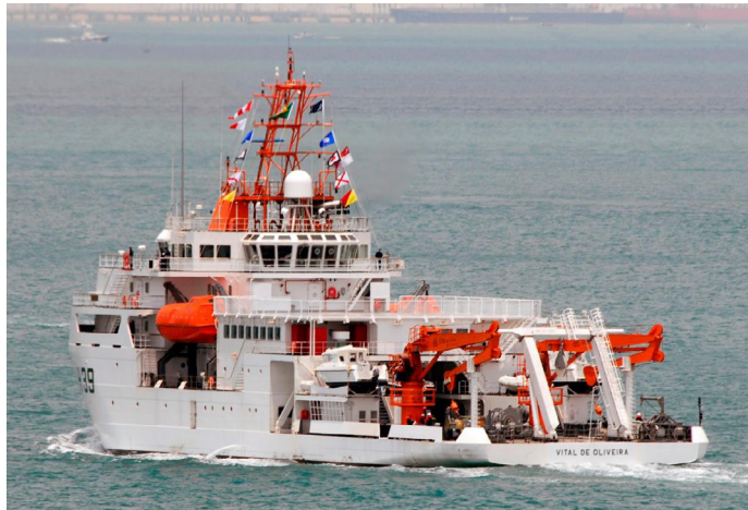
Fig. 1 Hydroceanographic Research Vessel "Vital de Oliveira" can conduct hydrographic surveys with its two hydrographic research boats and an ROV (Brazilian Navy).
