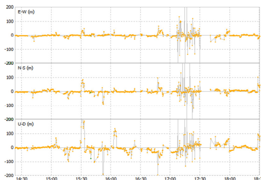
Fig. 17 Standard deviation as a function of time, for dual frequency positioning in Pracubinhas-PA.
