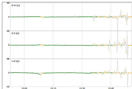
Fig. 21 Standard deviation as a function of time, for dual frequency positioning at Humaitá-AM.
