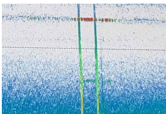
Fig. 12 The Mesobot (red horizontal target) confirmed to be directly in the scattering layer. At this point sampling is triggered assuring that eDNA samples were taken directly in the targeted layer.
