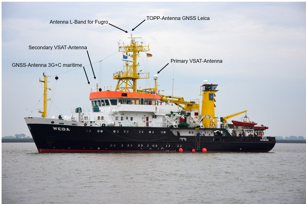
Figure 10. VWFS WEGA with the name and location of relevant antennas used for the September 2021 test cruises.
