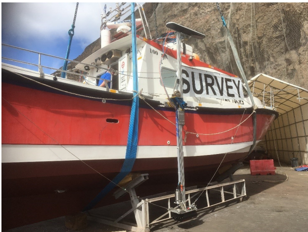
Figure 5 : Kongsberg 2040 mobilised to MV Enchanted Isle prior to lifting back in the water
