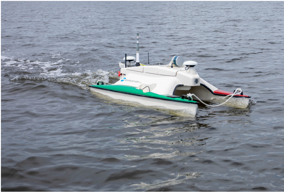
Figure 4: The SR-Surveyor M1.8 ( https://www.searobotics.com/products/autonomous-surface-vehicles/sr-surveyor-class ), developed and owned by SeaRobotics, a local Florida company, and used for a couple of our projects. Photo credit: Brianne Lehan.
