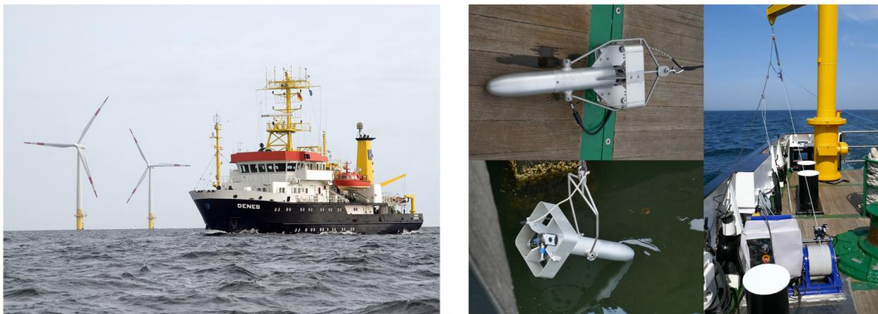
**Figure 2:** The BSH survey ship VWFS Deneb (left) and the newly installed (June 2020) AML Oceanographic MVP-30 underway profiling system (right).
