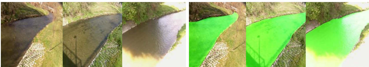
Figure 5: Successful river surface detection in over-/underexposed images (from Akiyama et al., 2020).
