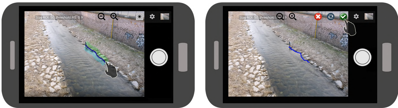
Figure 2: Visualisation of user interactions in OWL (from Elias, 2021). Left: pre-selection of the water line in the time-lapse sequence, Right: Acceptance / Rejection of the image-measured water line.
