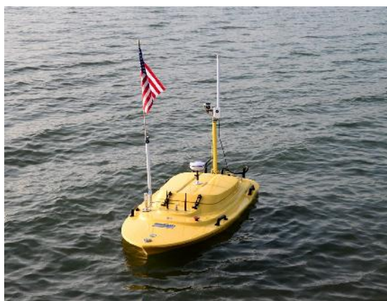
Figure 2a + 2b: The Technology Working Group learned about the uncrewed Z-boat, with multibeam sonar, as one option to choose from on surveying shallow waters for NOAA's coastal mapping program and to fill voids from topobathy lidar where waters are too turbid for full bottom coverage.
