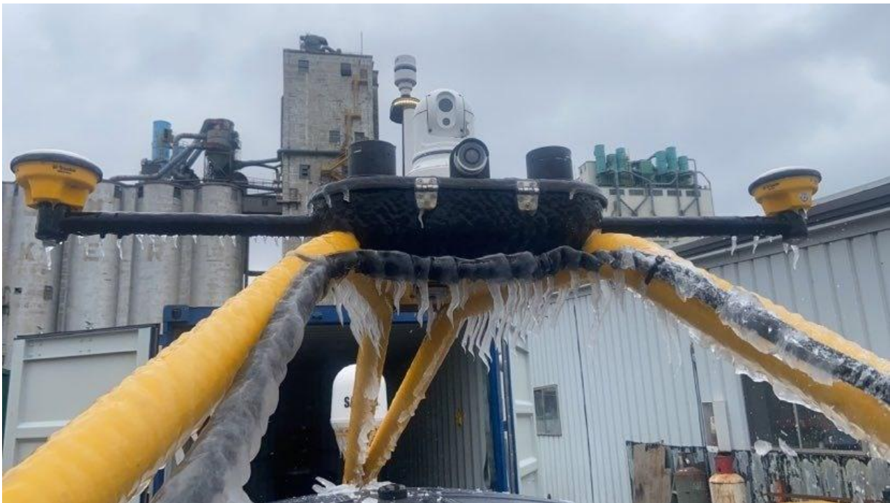
Figure 10: Ice formation on the gantry of XO-450 USV
