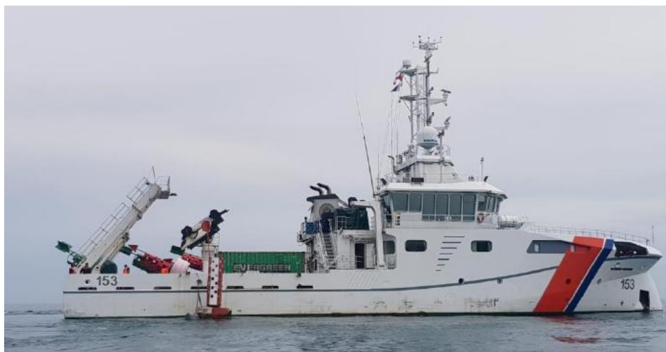
Figure 9. ARC Roncador installing the buoy safe water. Source: SHN
