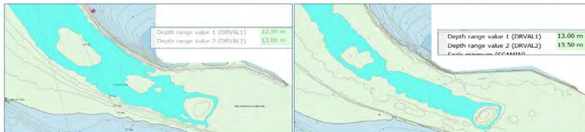
**Figure 7:** Contours based on re-gridded surface (left) and based on smoothed surface (right)
