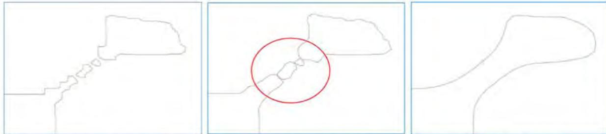
**Figure 6:** Contours based on Rolling Coin smoothing only (left), on Rolling Coin with contour generalisation (centre), on Rolling Coin and Laplacian smoothing (right)
