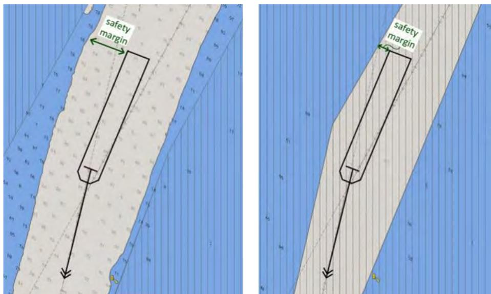
**Figure 2:** Differences in safety margins displayed on HDbENC (left) and on Harbour ENC derived from paper chart (right)
