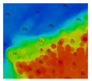
*Figure 4.* Application of the shoal expansion function to the re-gridded bathymetric surface
