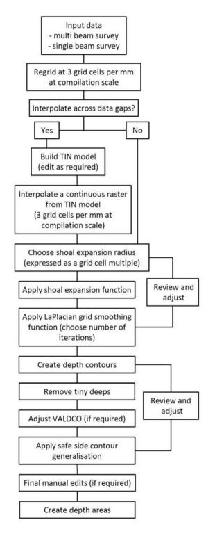
Figure 1. Flow diagram of the bathymetric feature creation method using CARIS BASE Editor tools
