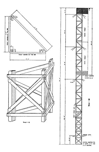
As shown by the accompanying drawing, the cross-section is a right triangle with sides 4, 4, and 5.66 feet. Here the utmost economy is realised for the usual stock lengths of material are easily divisible without waste. For example: 4 4-foot girders, or 2 5.66-foot girders and I 4-foot girder could be cut from a 16-foot  $2'' \times 4''$  board; 3 5.66-foot girders from an 18-foot  $2'' \times 4''$ , and I 5.66-foot and 2 4-foot girders from a 14-foot length.
