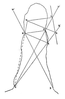
Next set the table up at the flag K, orienting on A. Then draw a long orienting line toward the flag N at any convenient place as kn. It must be kept in mind that the intersections k and n of this line with Ak' and An' are not the actual points K and N on the sheet, for K, the place of set-up, has not been located.
