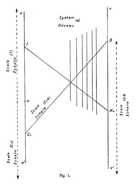
For a given value of  $C_0$ , B is joined to the graduation  $C_0$  on the scale  $(C_0)$ and this straight line is divided into  $\alpha$  by means of its intersections with the system  $(\alpha)$ . Thus a scale  $(C_0, \alpha)$  graduated according to  $\alpha$  is obtained.
