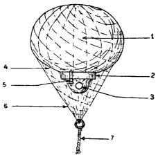
The *Pelt* consists of a canvas sphere 62 inches in circumference with a circular wooden base in which is a hole for securing the mooring rope. In this wooden base is fitted an ordinary non-return valve such as is used for the inner tubes of bicycle tyres and the sphere is inflated by means of the ordinary bicycle pump.
