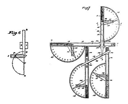
The mechanism whose principle is illustrated in Figure 6, being applied at the end-ordinates of the square forming the boundary of Figure 4, provides for determining the line of the graph of equation (10), or (11), or (12) by means of the fiducial edge of the bar or ruler pivoted to the head of one of the pair of members QB shown in Figure 6 and sliding over a support at the head of the other.
