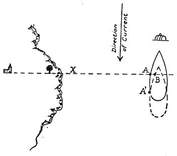
Thus, in the annexed figure, at the commencement of the observations the ship was in the position shown by the firm line and the transit line AX was observed from the point A.
