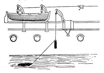
water may begin a series of swinging movements, each successive movement increasing in range in proportion with the shortening of the distance between lead and block.
