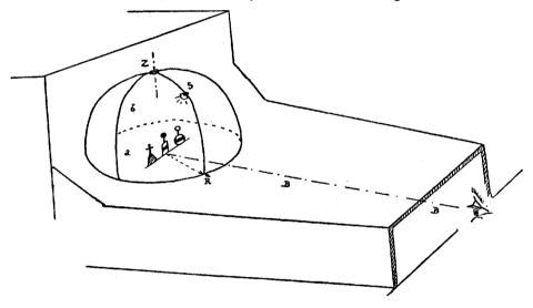
One quarter of a sphere representing the celestial concave (restricted to the plane of the horizon), as it is called in astronomical navigation, will serve as the lighted field for tests in the interior of a container of a suitable shape blackened inside, in the centre of which may be placed small models, reduced to a predetermined scale, representing buoys and giving them their actual shapes and not only their silhouettes.
