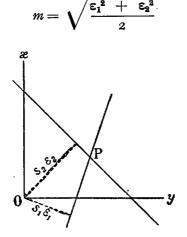
Assume that m is equal to the quadratic mean of the deviations of the bearings taken with respect to their mean values. If O is the point determined
