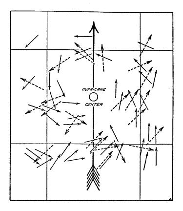
The observations in attached figure show the deviation of swells to the right of the wind; that is, an observer standing with his back to the wind would find the swells moving off to his right.
