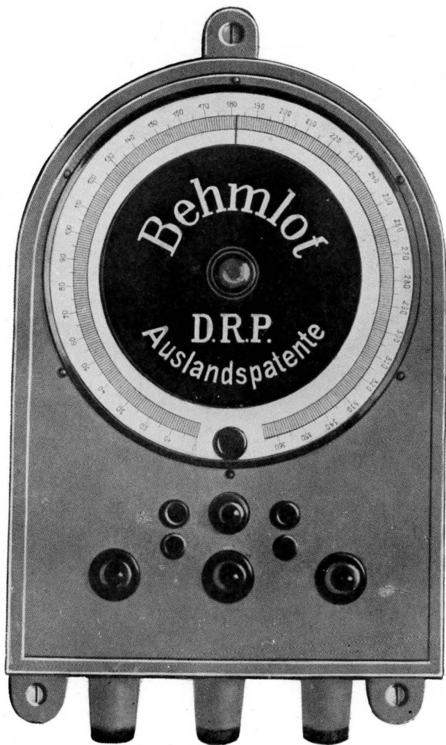
Fig. 31. — Behm Sounding machine with indicator. Patented in Germany and in Foreign countries.
