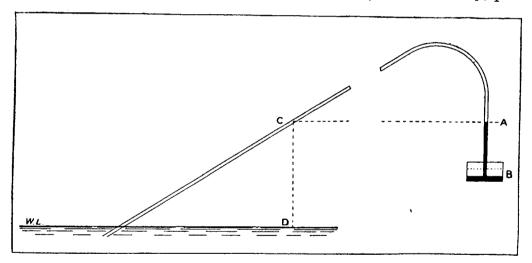
vided the highest portion of the tubing is not more than about 30 feet (9 m.) above the level of the sea.
