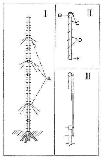
$7^{\circ}$  When all is ready, attach the end of the falls from the davit to the next tube to be fitted in place. The falls should be attached to the tube sufficiently close to the sleeve so that the tube will be drawn up vertically with the sleeve up.
