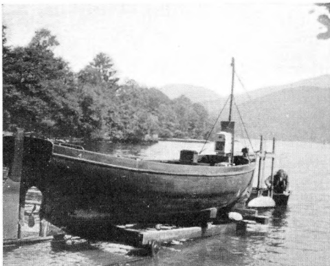
Launch fitted with recorder and outboard Oscillators at Lake Windermere.
