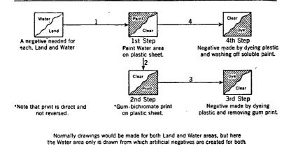
A further use of the plastic sheet in this plant has been the production of duplicate negatives, which can be accomplished without the usual intermediate step of first making a positive.
