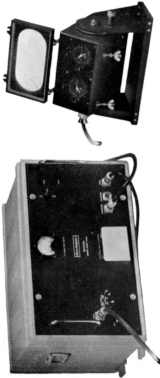
FIG. 2 Photo showing the special Decca survey receiver.
