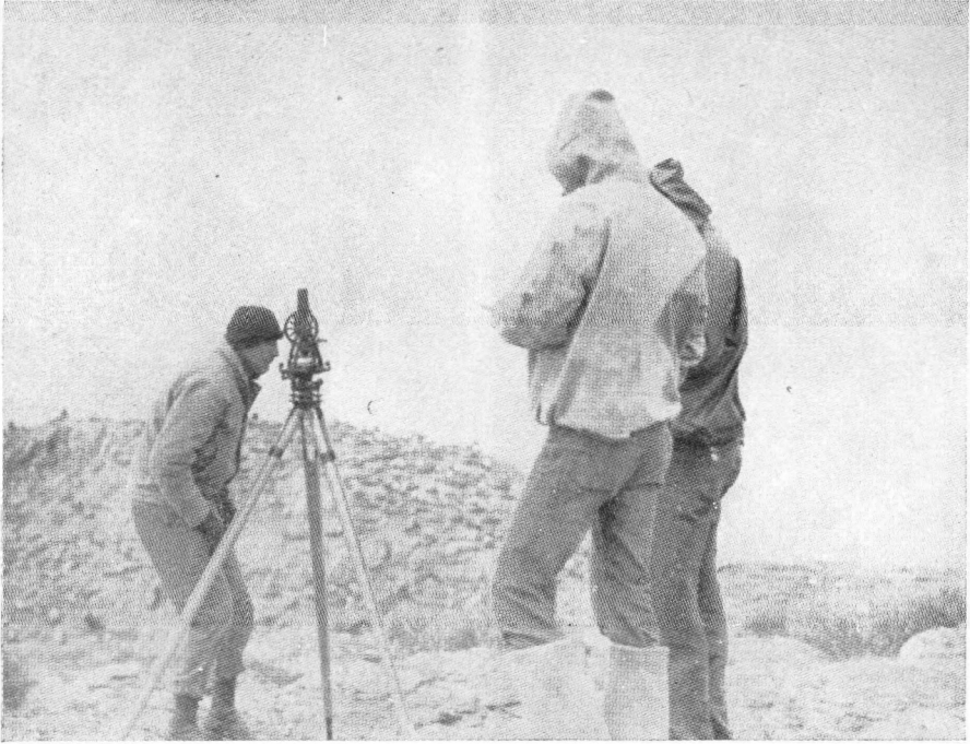
Fig. 11. — Making magnetic observations with a transit magnetometer
