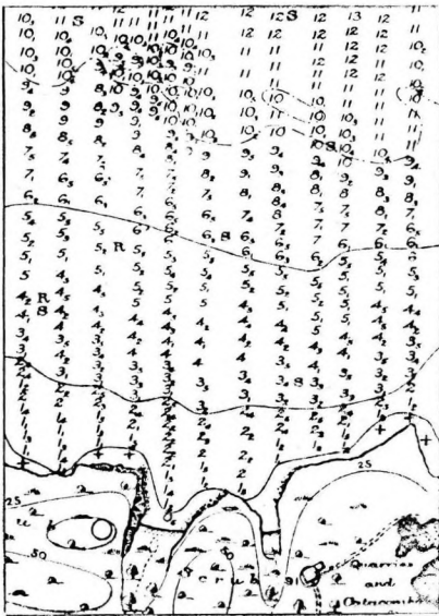
Fig. 6. — A portion of a chart compiled from a survey (left) using sonic sounding methods.
