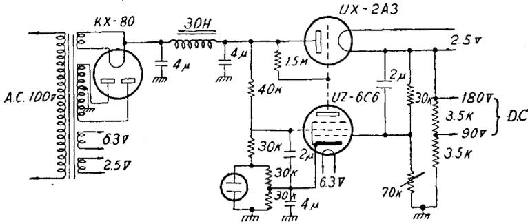
Fig. 6. — Schematic circuit diagram of D.C. stabilizer
