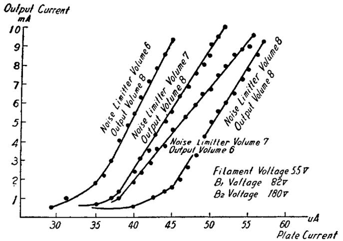
Fig. 5. — Relation between the output and the plate current.
