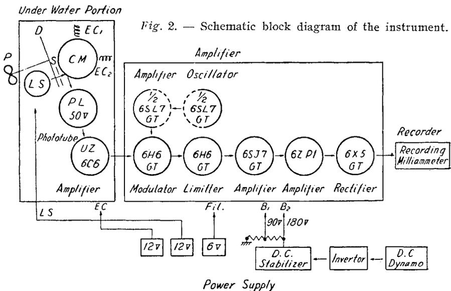
Fig. 2. — Schematic block diagram of the instrument.
