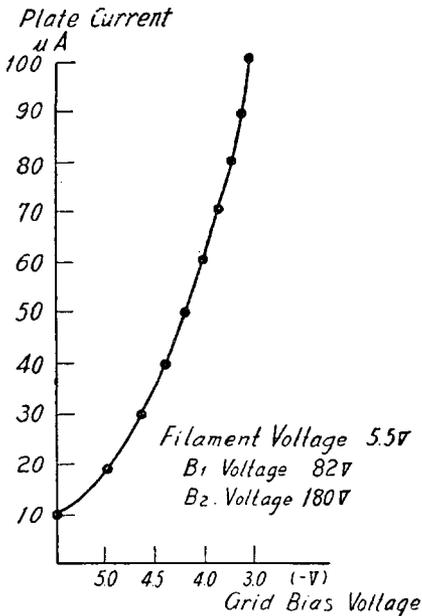
Fig. 4. — Relation between the plate current and the grid bias voltage.
