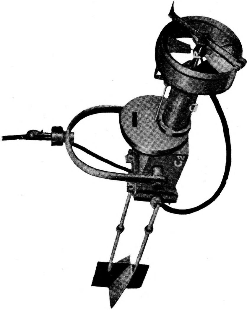
Fig. 1. — The under-water portion of the current meter, which sends photoelectric signals.
