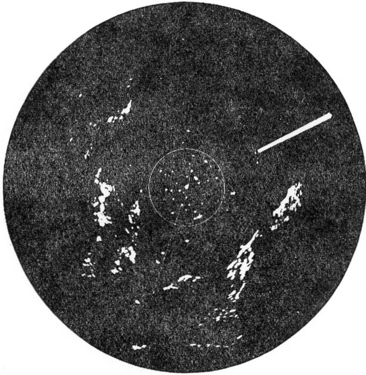
Fig. 3. A modern PPI photograph of the Thames Estuary. Note the racon response on the Tongue light-vessel and absence of the boom defence shown on the mosaic.
