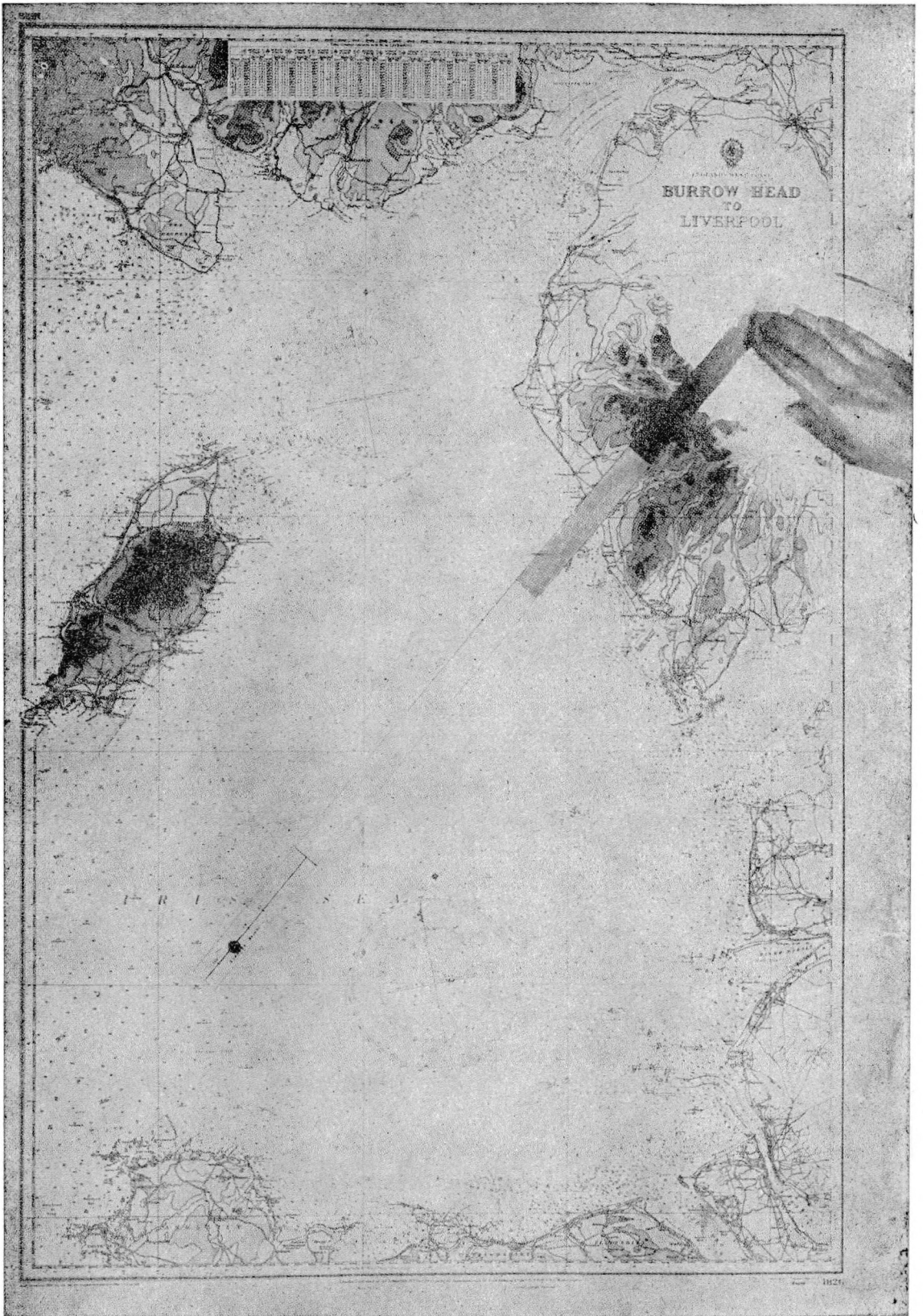
Frontispiece. Admiralty Chart 1826. A graded strip pinned, through the 75-ft. scanner height mark, on to the D.R. position shows that only the mountain tops in Cumberland would be above the radar horizon at this range.
