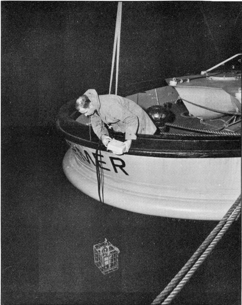
Fig. 7. — The inductive conductivity temperature indicator being lowered over the stern of the Marmar . This device measures the temperature and salinity instantaneously for any required depth.
