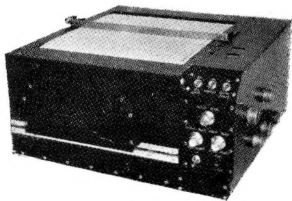
LORAC ACTRAC UNIT FOR THE CONTINUOUS PLOTTING OF POSITION.
