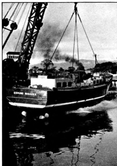
FIG. 8. — The stripped hull of M. L. Edmund Rhoades is lowered by crane into the waters of Lake Nyasa at Chipoka, at the end of her journey by sea and rail from England.
