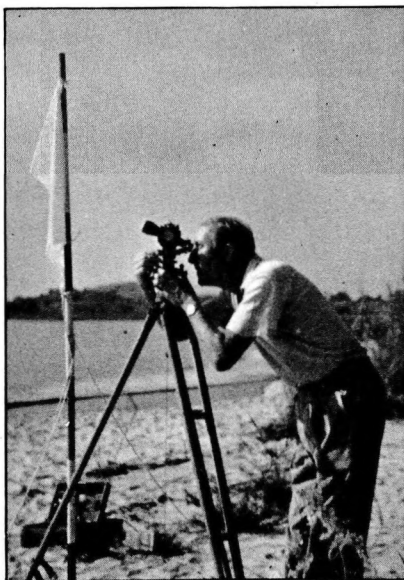
FIG. 10. — The author observing the sun for azimuth at the end of one of the beach base lines.
