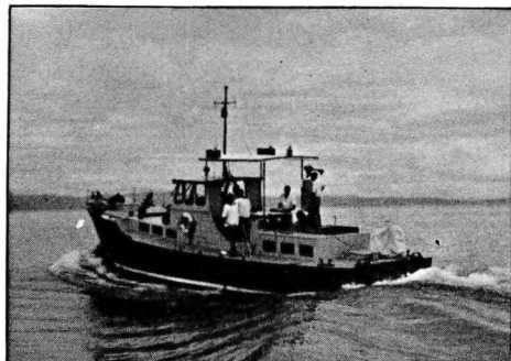
FIG. 4. — M.L. Edmund Rhoades , 46 feet, powered with two Gardner 6-cylinder diesel engines to give a speed of 10 knots.
