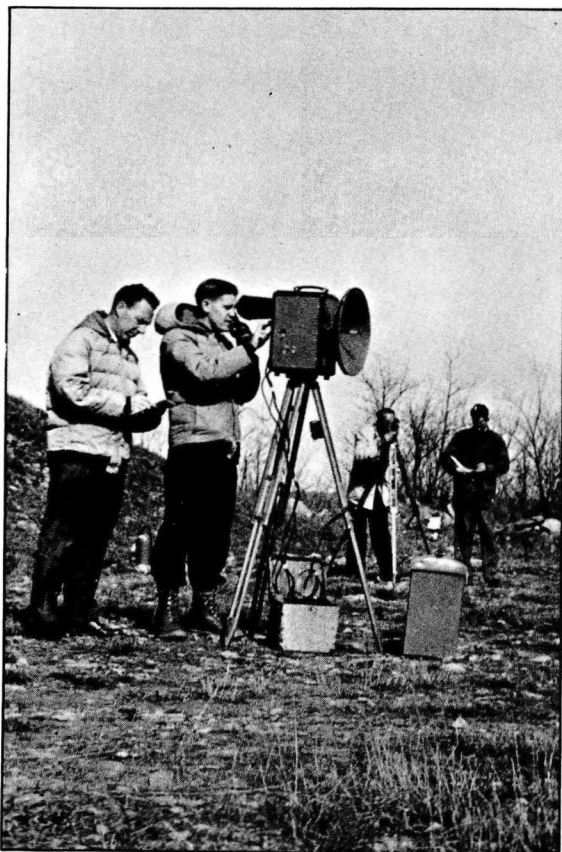
FIG. 2. — Instruction in the use of Tellurometer and Theodolite is part of a training programme in modern surveying methods.
