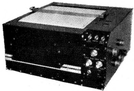
LORAC ACTRAC UNIT FOR THE CONTINUOUS PLOTTING OF POSITION.
