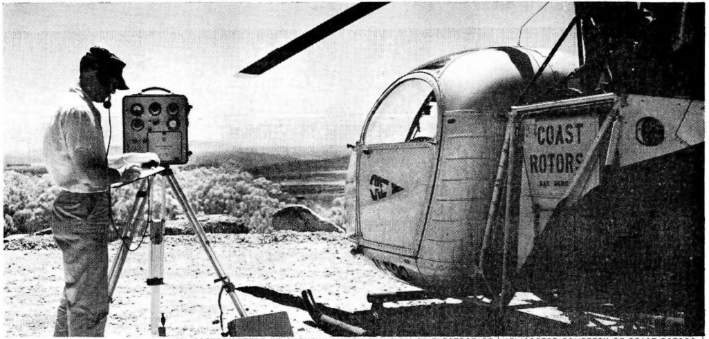
HELICOPTER SPEEDS UP SURVEYING WITH CUBIC DM-20 ELECTROTAPE (HELICOPTER COURTESY OF COAST ROTORS.)
