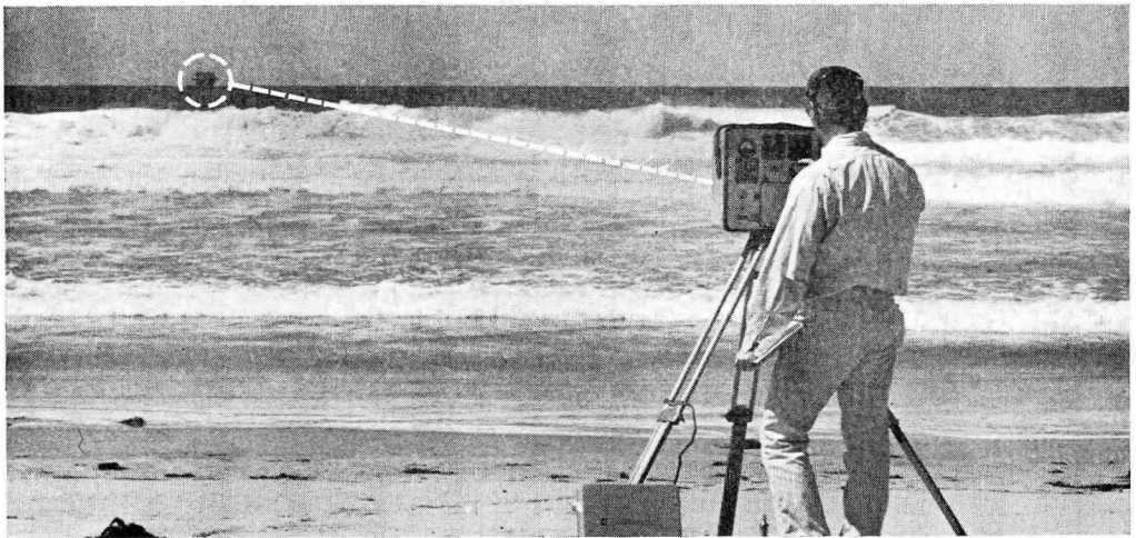
CUBIC DM-20 ELECTROTAPE QUICKLY PINPOINTS LOCATION OF OFF-SHORE INSTALLATIONS.
