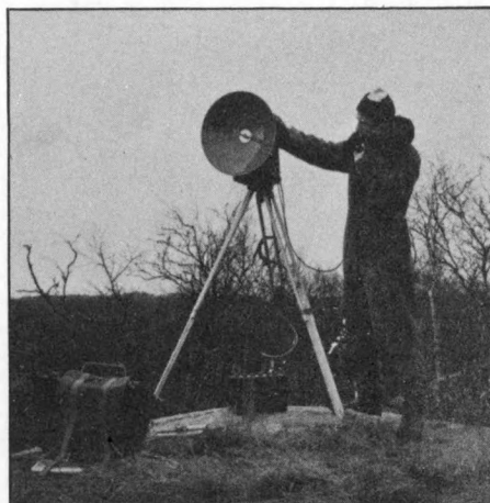
FIG. 8. — A Hydrodist shore station. The attendant is just talking with the ship.
