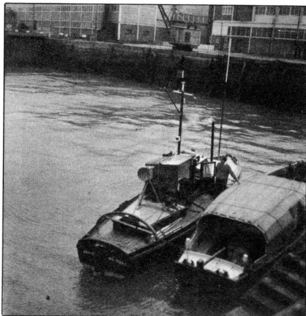
Motor Tug Sally with tellurometer secured abaft the wheelhouse and plotting table.
