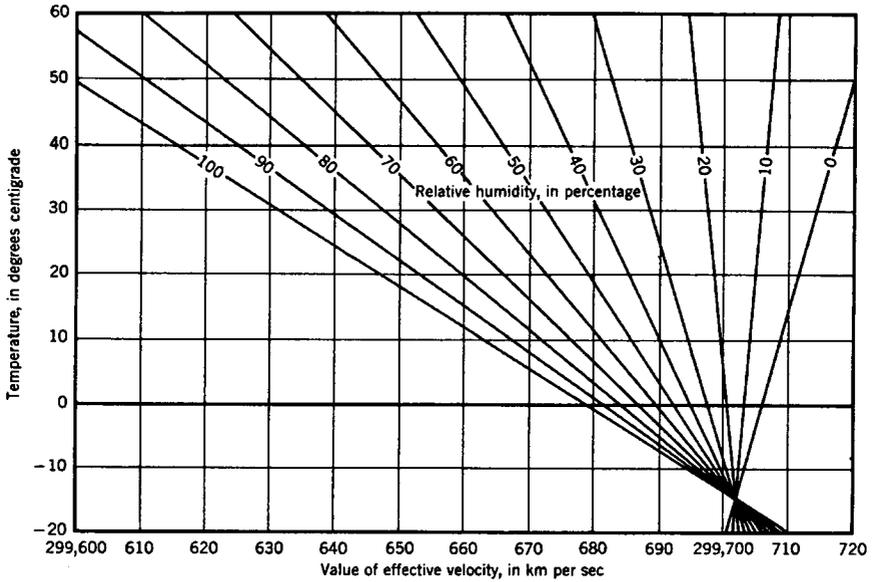
FIG. 14. — Effective velocity of propagation.
