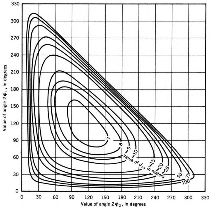
FIG. 7. — Solution of  $d_r$  in terms of angles  $2\varphi_1$  and  $2\varphi_2$ .
