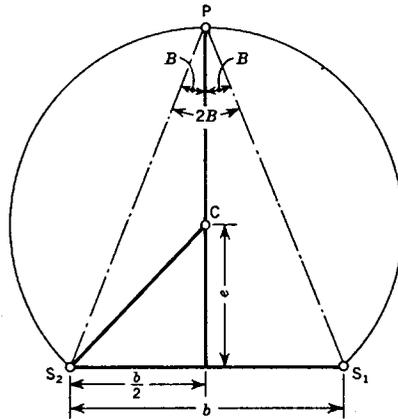
FIG. 4. — Center of arc of constant angle.
