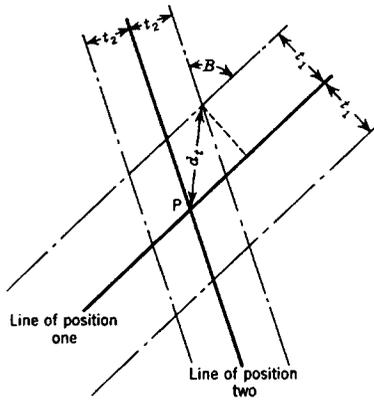
FIG. 3. — Derivation of the error of position.
