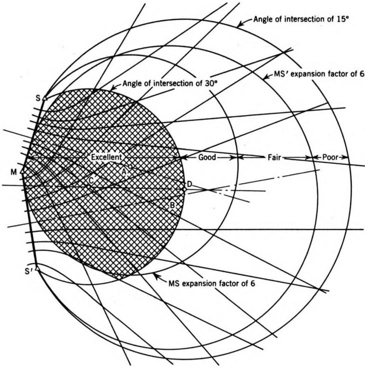
FIG. 6. — Typical reliability diagram, hyperbolic triad.
